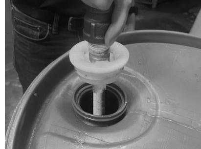
2. Place the GMP base on top of the 55-gallon drum with reducing valve facing the dip tube assembly. Install and tighten drum clamp to secure GMP to the 55-gallon drum.
