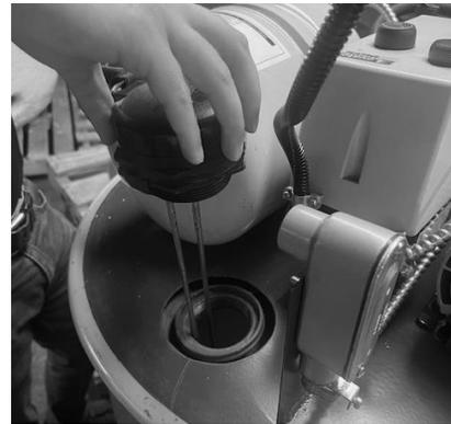
4. Install the pump suction hose onto the dip tube.
