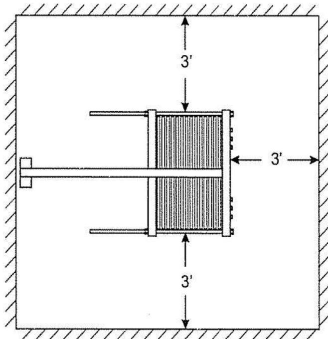
The foundation for the heat exchanger must be level and firm enough that no settling occurs which could put forces and strain on the piping connected to it.
