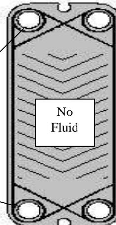
Depending on the number of passes a plate heat exchanger may have, the connection location may vary. Since all of the heat exchangers are parallel or same side flow, all connections for one fluid will be on the right side and the opposing fluid on the left side.
