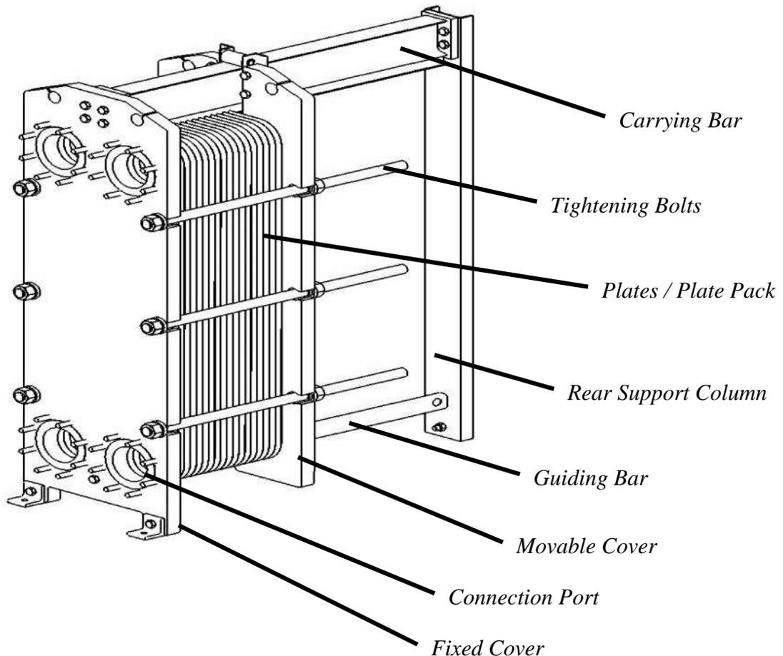
The frame is made up of thick steel pressure retaining parts, the *fixed cover* and the *movable cover*, that when pulled together with the *tightening bolts* form the pressure retaining structure for the *plates / plate pack*.
